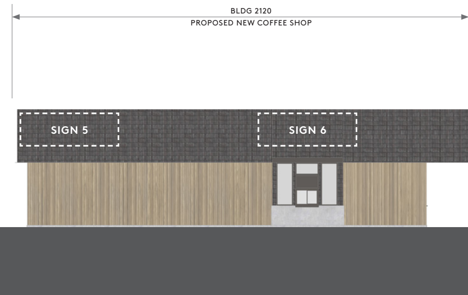
WEST ELEVATION FACADE SURFACE AREA: 48'-7" X 9.5" + 54'-0" X 9.5" + 12' X 6' = 1,000 SF 1,000 SF X .20* = 200 SF 200 SF MAX. ALLOWABLE SIGNAGE AREA
