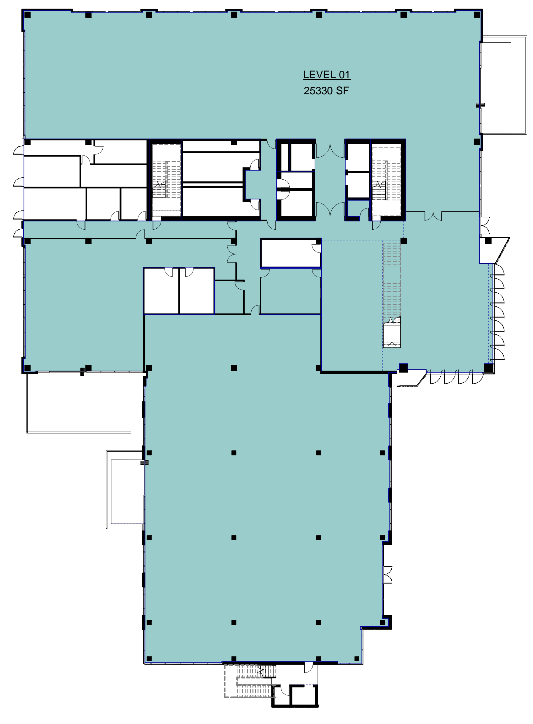
NET FLOOR AREA - LEVEL 01 SCALE: 3/64" = 1'-0" ①
