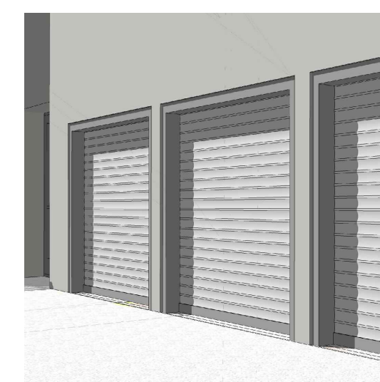
9 TYPICAL METAL ROLL-UP TRASH ROOM DOOR
