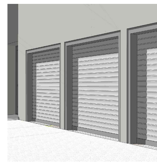
12 TYPICAL METAL ROLL-UP TRASH ROOM DOOR
